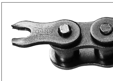
① Static fracture Applying load to a link plate beyond its breaking load will cause it to stretch and then break.
