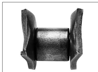
③ Offset link plate fatigue breakage Offset link plates are bent at the center, and the resulting concentration of stress at the bend can cause a fatigue break. Avoid using offset links in high-stress applications.
