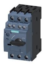
Circuit breaker 10 A A-release 7...10 A, N-release 130 A, for motor protection, class 10, screw connection, standard switching capacity w. transverse AUX. switch 1 NO + 1 NC
